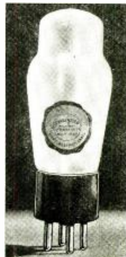
Battery-type ballast. (No. 463) This device eliminates rheostats.
