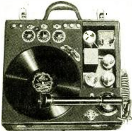
Fig. B, left A view of the amplifier, mixing controls, phono-turntable, pickup, and all in one side of case.
